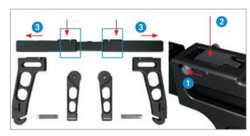
After disassembly, clean the rails, arms and threaded tubes manually, e.g. by using a brush. The springs in the upper arm at button should be cleaned too. If necessary, broken or damaged parts should be exchanged.
